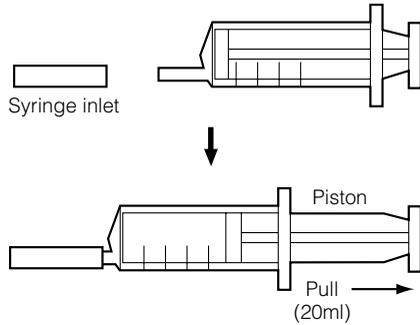
3 Insert the tube securely into the syringe inlet with the arrow pointing away from the pump. Inject the sample collected in the syringe into the detector tube in 2 minutes (for No.100B) or 20 seconds (for No.2HT), and read the indication.
