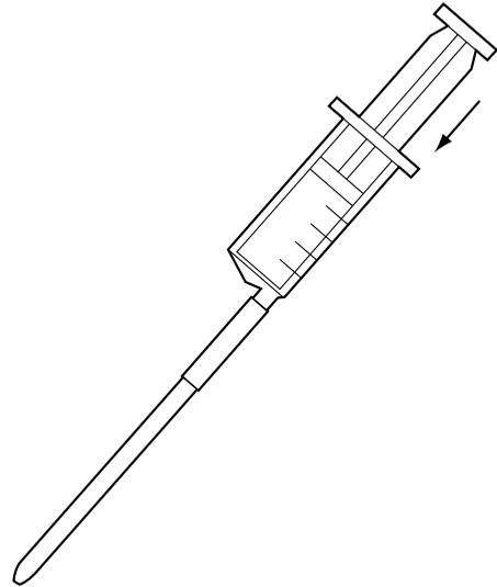
2 Break off both ends of a detector tube (No.100B for No.601 syringe or No.2HT for No.611 syringe) by using the tube tip breaker.
