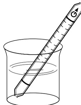
▣ **Airtec tube - Compressed breathing air detector tubes**
